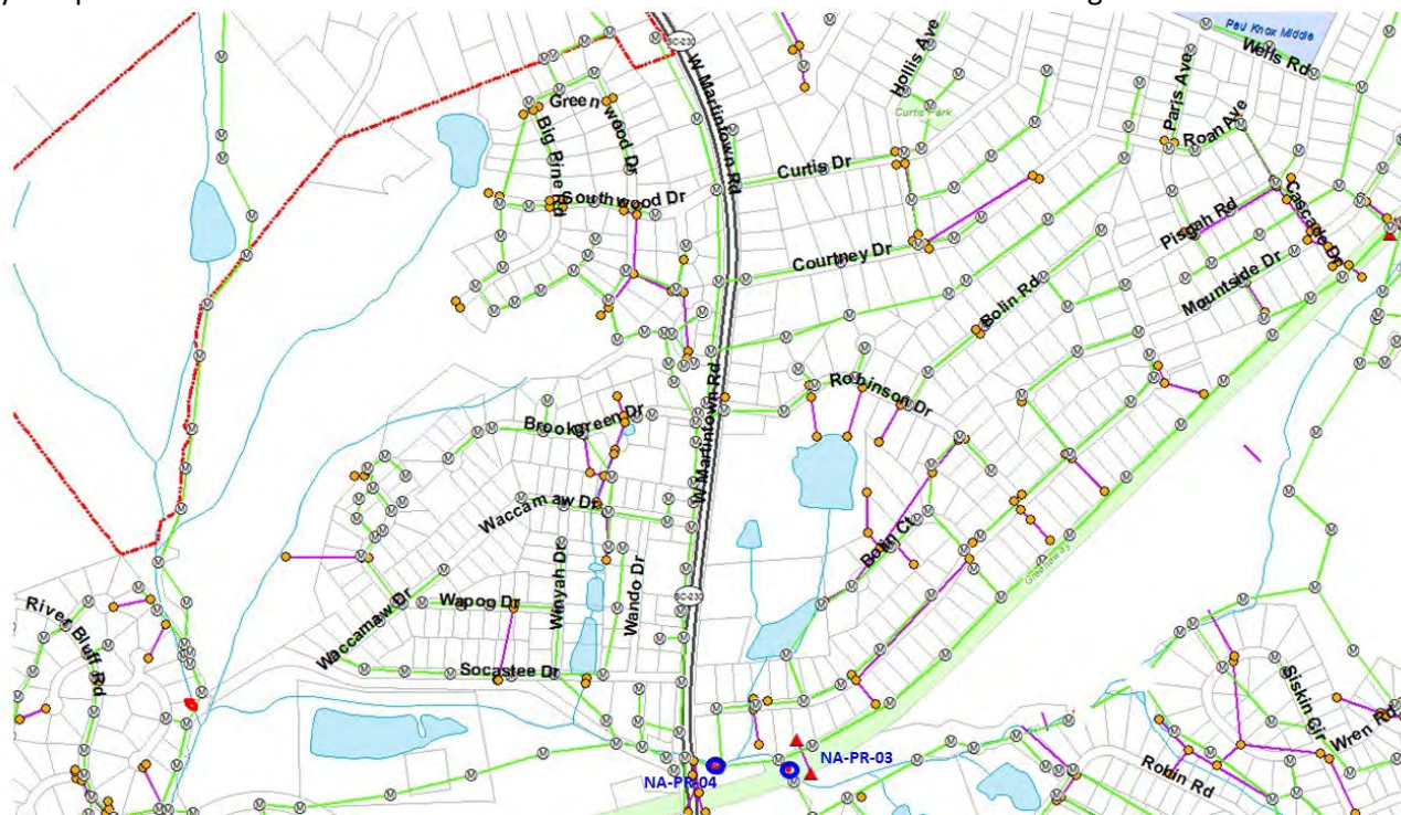
Figure 16: GIS Map of TMDL Monitoring Location NA-PR-03 and NA-PR-04 with Infrastructure (Green lines with manholes = Sanitary Sewer, Pink lines with orange manholes = Storm sewer)
