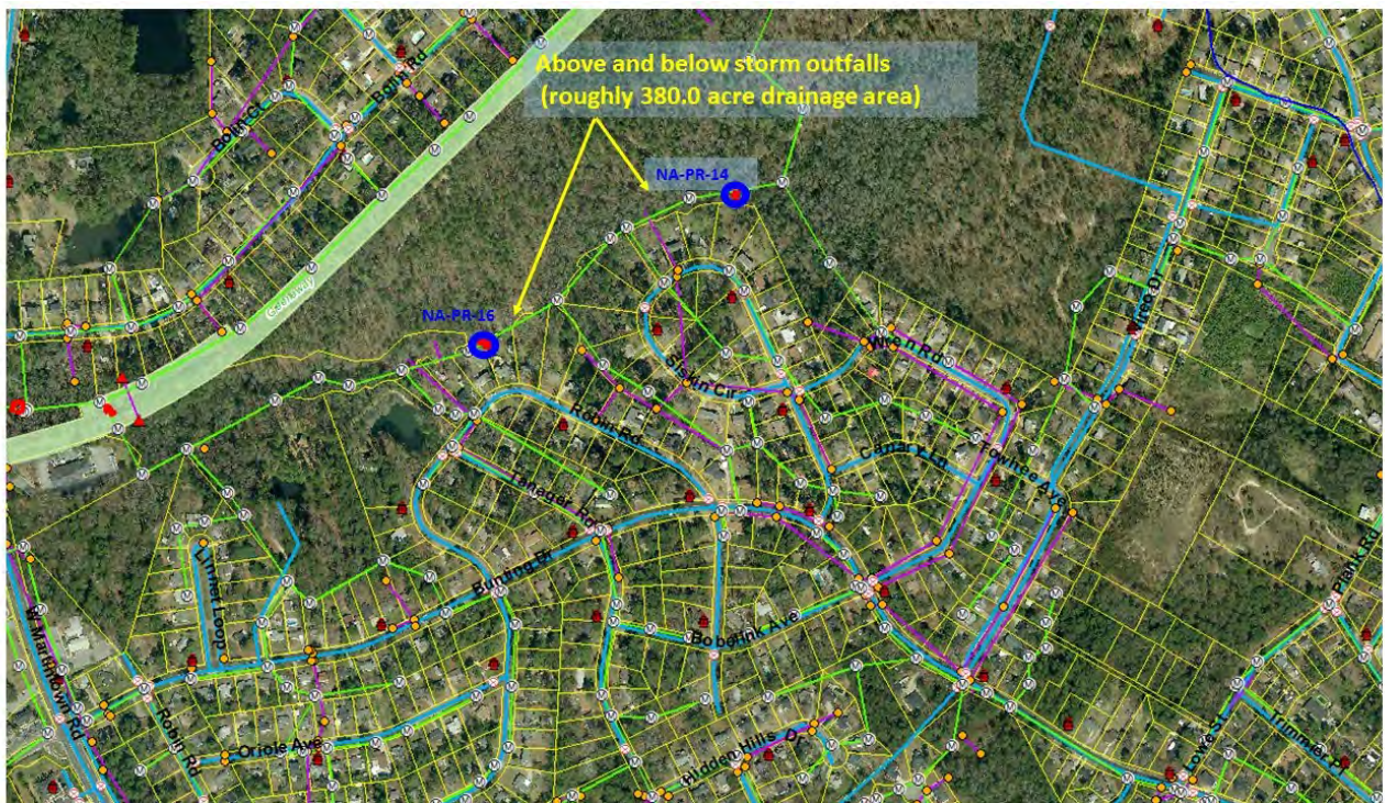
Figure 19: Aerial Image of TMDL Monitoring Location NA-PR-16 and NA-PR-14 with Infrastructure (Green lines with manholes = Sanitary Sewer, Pink lines with orange manholes = Storm sewer)
