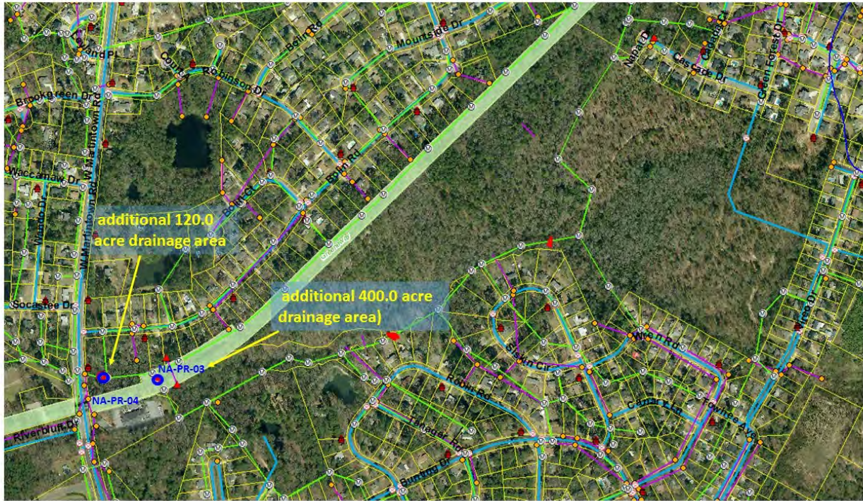
Figure 17: Aerial Image of TMDL Monitoring Location NA-PR-03 and NA-PR-04 with Infrastructure (Green lines with manholes = Sanitary Sewer, Pink lines with orange manholes = Storm sewer)
