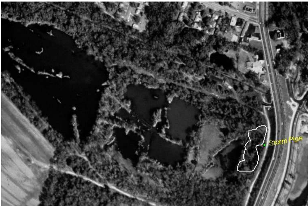
Figure 2. Pools one through ten and the location of the stormwater pipe that delivers most of the stormwater runoff from the upper regions of the drainage basin.
