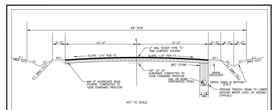
NOTES: 1. TOP OF 12" SUBGRADE TO BE MIXED IN PLACE AND COMPATED TO 100% STANDARD PROCTOR.
