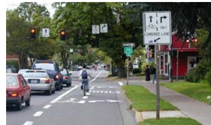
Shared bike right turn lanes require signage as well as pavement markings.
