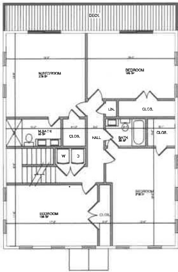
PROPOSED 2ND FLOOR PLAN SCALE: 1/4" = 1'-0" (AS SHOWN)
