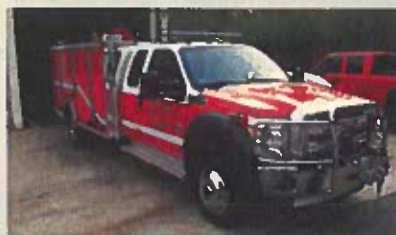
Rescue 2 2011, Ford 550 250 gpm pump 250 gallon 2036
