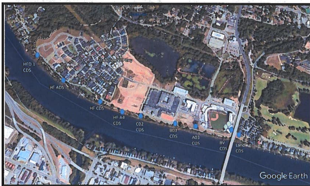
Figure: 4.1 North Augusta Riverfront development underground stormwater treatment unit locations.
