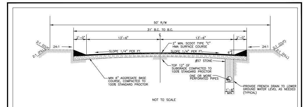
NOTES: 1. TOP OF 12" SUBGRADE TO BE MIXED IN PLACE AND COMPATED TO 100% STANDARD PROCTOR.
