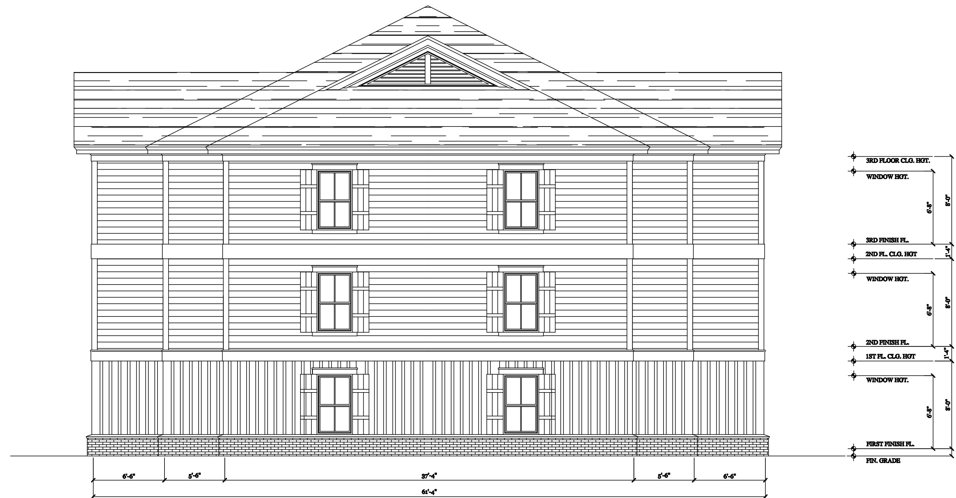
SIDE ELEVATION SCALE: 3/16" = 1'-0"
